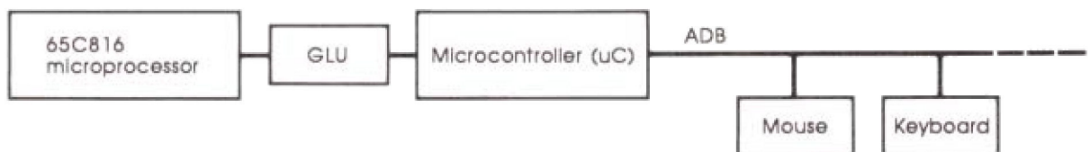
Figure 9-1 Apple DeskTop Bus components
